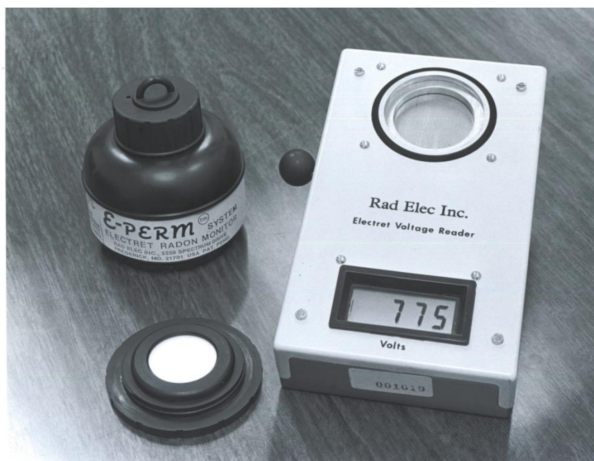
Figure 7. Components of EIC for radon measurements; top left: radon EIC, top right: electret voltage reader, bottom left: electret in open mode.
