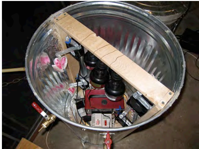
Figure 6 - 114 liter Thoron Chamber using Aladdin mantles & fans
