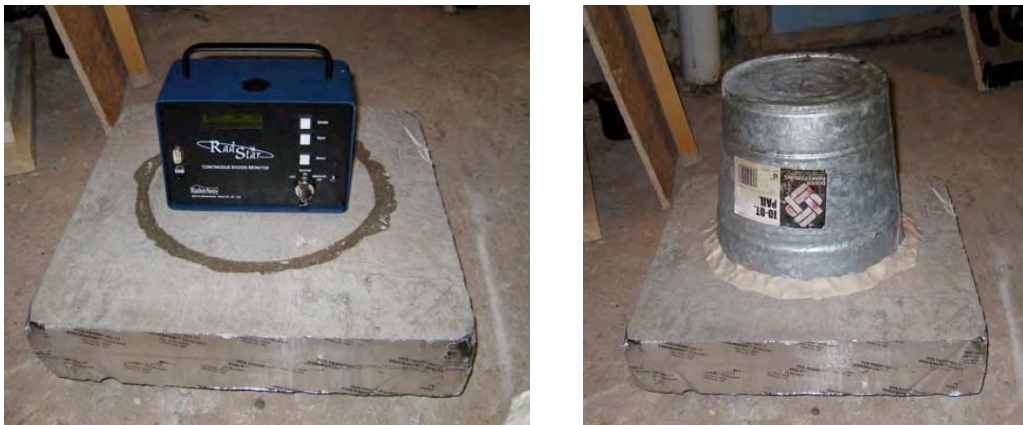
Figure 11 – RS800 sealed under 9.6 Liter Accumulator for Mixed Slab
