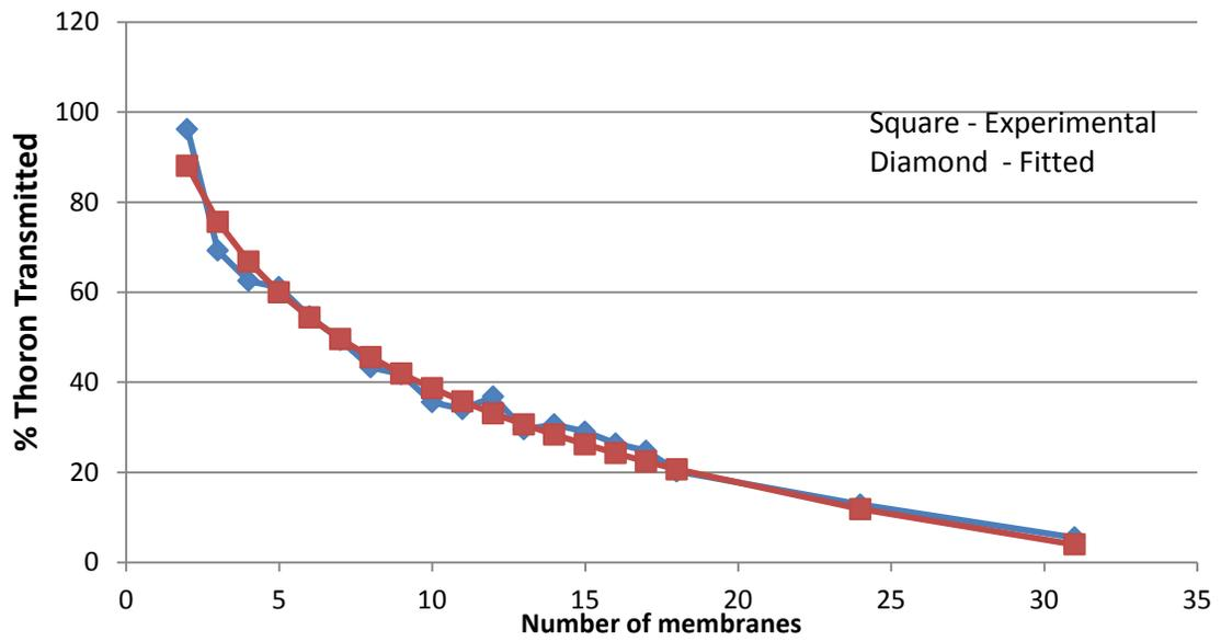
Figure (2): Percent thoron attenuation (experimental and regression fitted) for the stated number of Tyvek membranes
