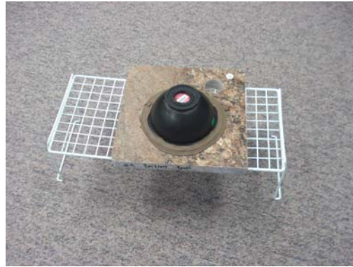
Fig 1b Deployment of the Radon Flux Monitor
