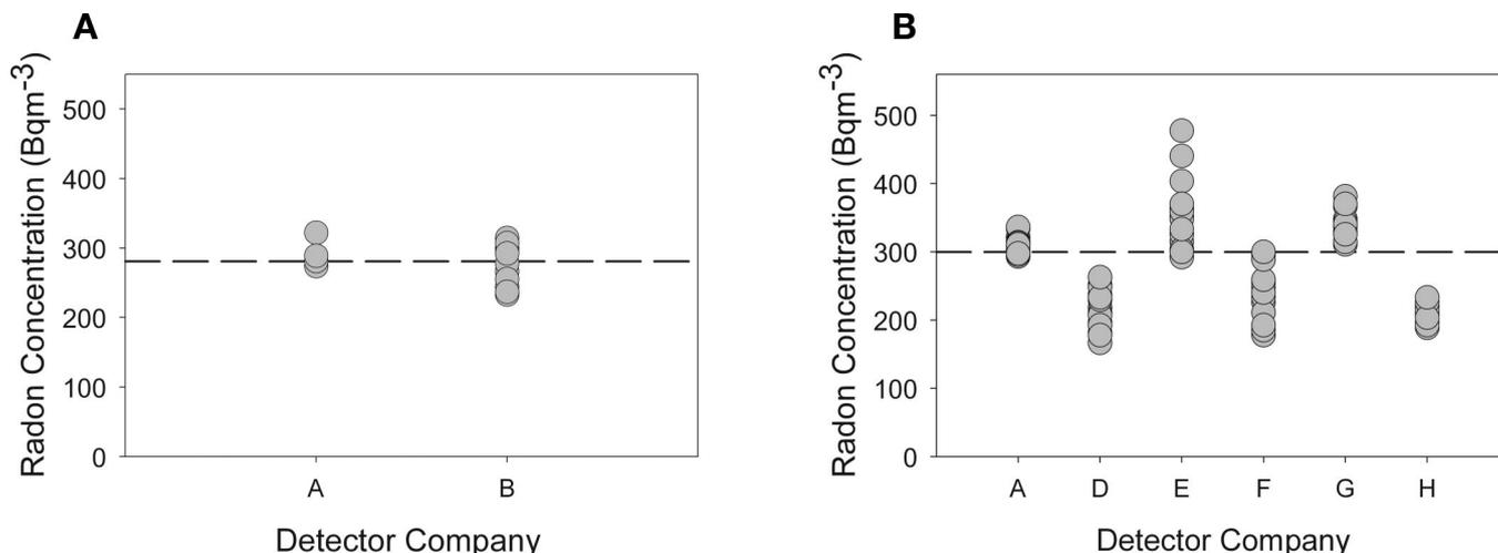
**Fig. 2.** (a) Comparison of the fifteen detectors from Company B and four electret ion chambers (Company A) as compared to the radon reference concentration (dotted line) obtained from the continuous radon monitor for the 3-d measurement period; (b) Comparison of the fifteen detectors from Companies D, E, F, G, H and fifteen electret ion chambers (Company A) as compared to the radon reference concentration (dotted line) obtained from the continuous radon monitor for the 4-d measurement period.
