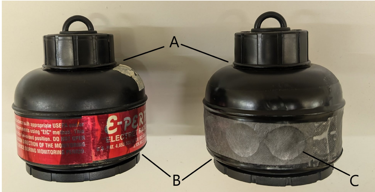
Figure (4): Potential entry points for radon with the chamber in the Off Position. E-PERM S chamber on the left, RT chamber on the right. A is under the cap, B is through the threads where the electret is screwed in, C is through the Tyvek-covered pores on the body of the RT chamber.
